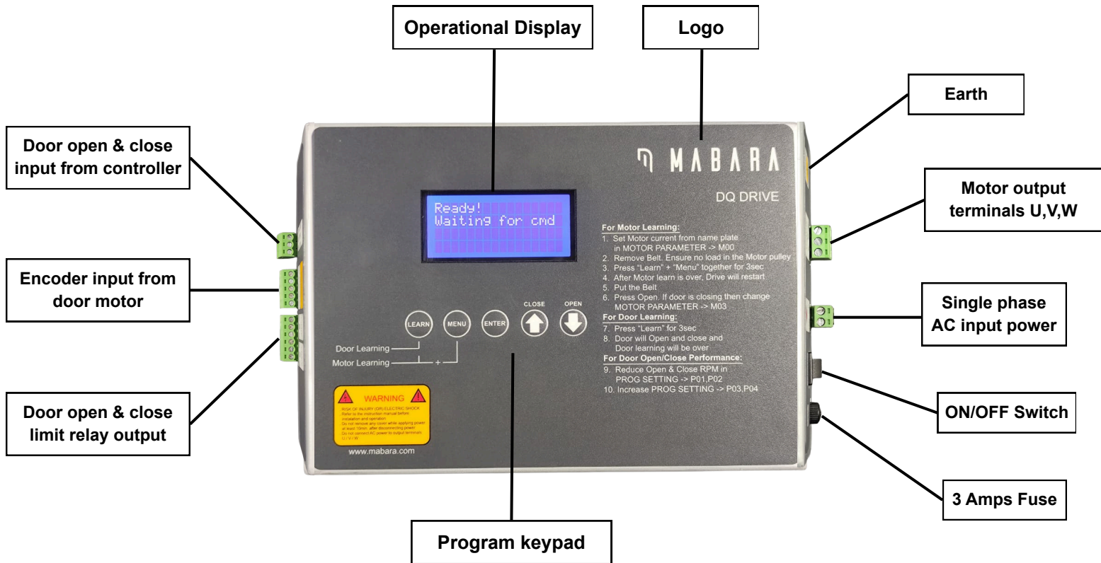
Figure 2-2 Structure of the MDDPM - DQ DRIVE
